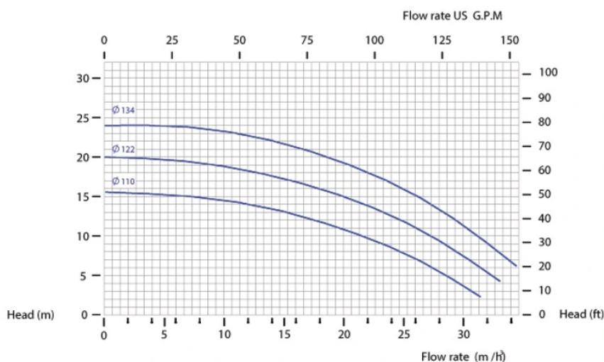
The curves and performance values refer to pumps with free delivery outlet with water at 20 °C, and two poles motor 50 Hz
